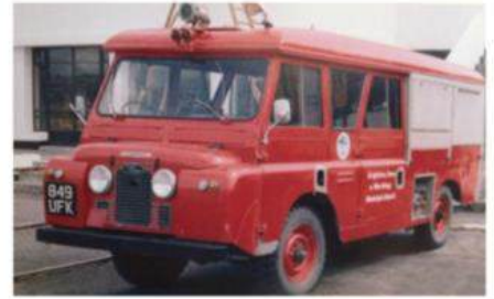
The 1961 prototype became 849 UFK and entered service with a municipal airport. The awkward shape of the side window between the doors was made necessary by using a standard front door sidescreen for the rear side door. The front wings were moulded from GRP, and in this case (as on a few later vehicles) have a distinctive curved feature; its purpose is unknown. (Unknown copyright)
