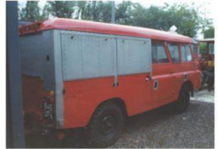
The 1961 prototype became 849 UFK and entered service with a municipal airport. The awkward shape of the side window between the doors was made necessary by using a standard front door sidescreen for the rear side door. The front wings were moulded from GRP, and in this case (as on a few later vehicles) have a distinctive curved feature; its purpose is unknown. (Unknown copyright)
